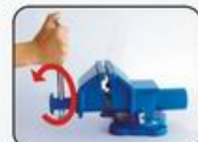
1. To open, turn handle one full turn to the left
